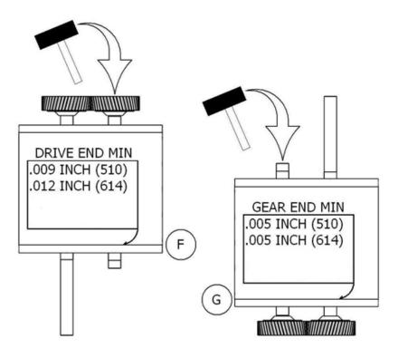
Fig. 13 Checking Minimum End Clearances
